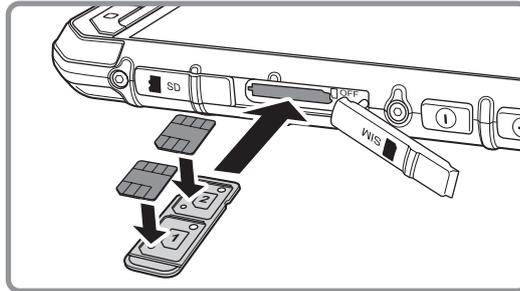
4. Insert the SIM tray into the SIM card slot.
